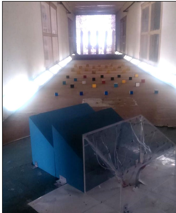
Fig 7: Three-span north-light roof building model inside the wind tunnel at 135° wind incidence angle
